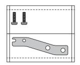
Kit consists of mounting plate and 2 self-tapping screws AC-EM-059-1  $\,$
