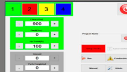
**Multi-Station:** Multi-Station is an option that allows the operator to insert more than one fastener in a program. Each station can be configured to have its own individual Force, Dwell Time and Up Travel.
