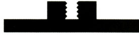
Zinc plated Mild Steel hexagonal nut on a blind 19mm diameter base plate
